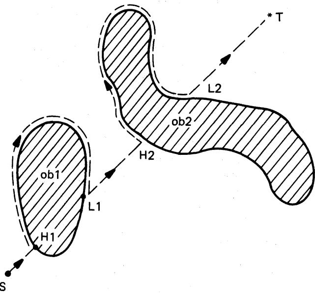
Figure 4. Automaton's path (dotted line) under the algorithm Bug2.
