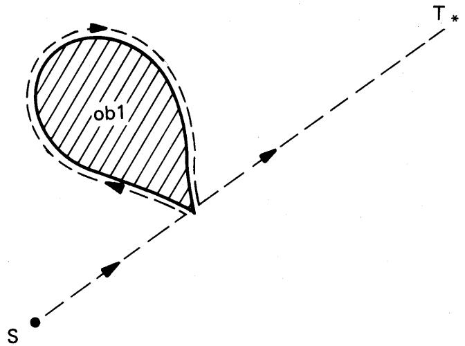
**Figure 7.** A case when, under the algorithm Bug2, the automaton will have to make almost a full circle around a convex obstacle.
