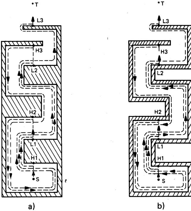
**Figure 5.** Automaton's path around a maze-like obstacle (in-obstacle position) under the algorithm Bug2. In terms of path complexity, both obstacles (a b) are the same, whereas for (a) the straight line ( $S, T$ ) crosses the obstacle 10 times,  $n_1 = 10$ , and for (b),  $n_1 = 16$ . At most, the path passes one segment (here ( $H1, L1$ )) three times; that is, there are at most two local cycles.
