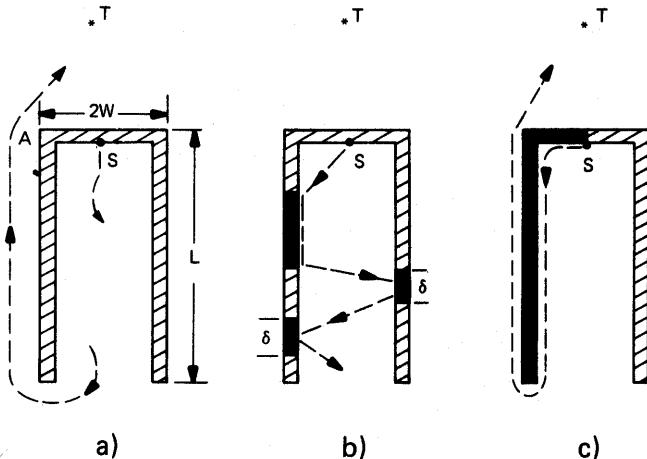
**Figure 1. Illustration for Theorem 1. Actualized segments of the maximum obstacle are shown in solid. S — Start point, T — Target point.**
