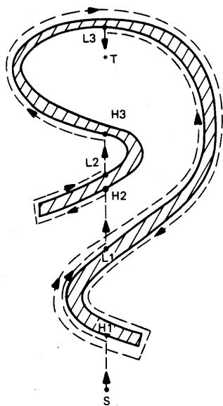
**Figure 6.** Automaton's path in case of an in-obstacle position; here  $S$  is outside the obstacle, and  $T$  is inside.
