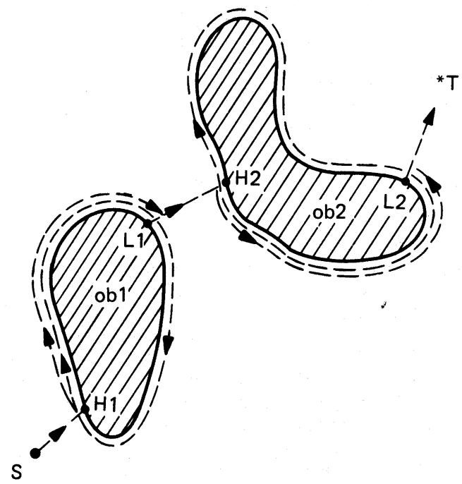
**Figure 2. Automaton's path (dotted lines), algorithm Bug1. ob1, ob2 — obstacles; H1, H2 — Hit points; L1, L2 — Leave points.**
