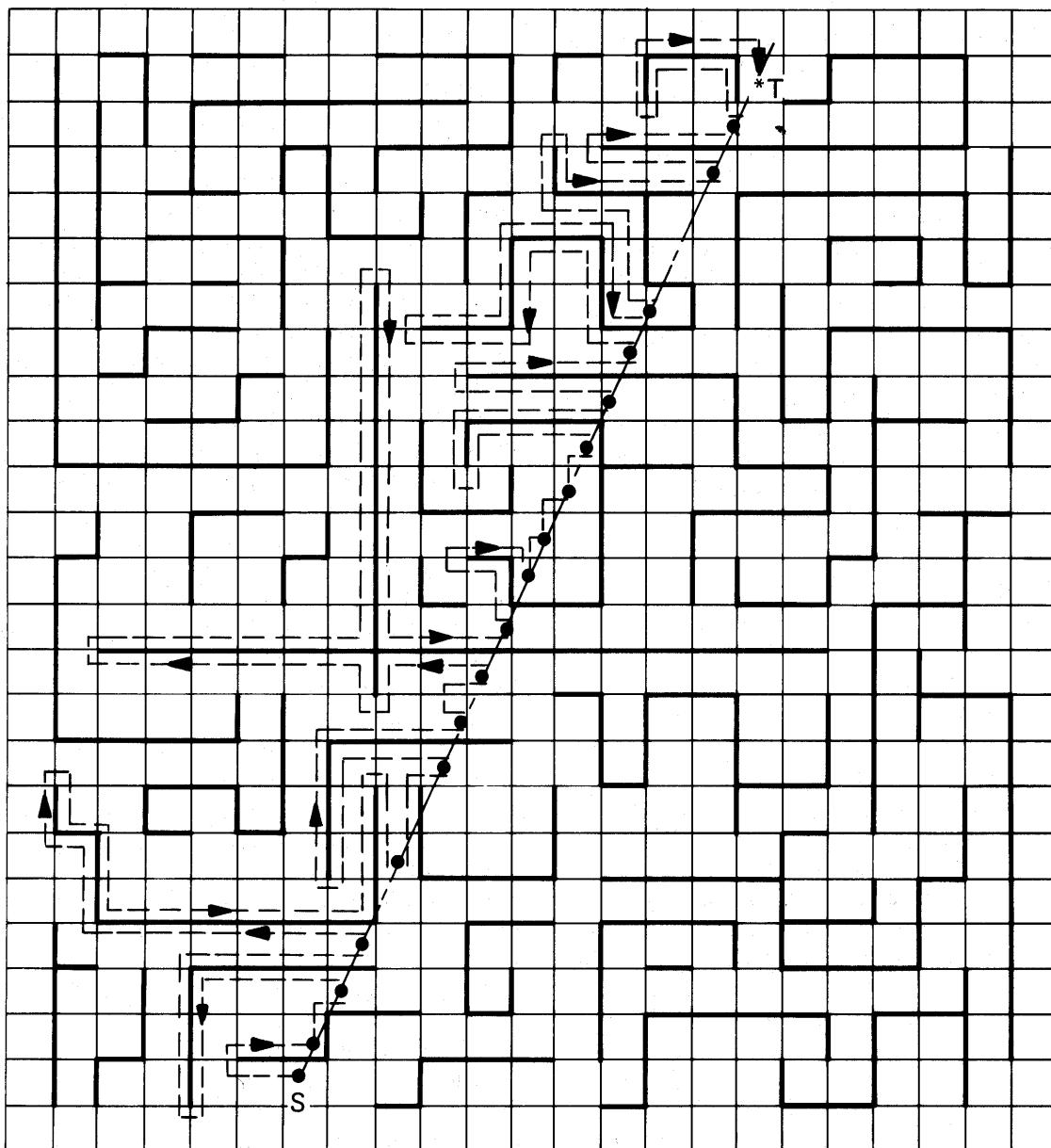
**Figure 11. Example of a walk in a maze using Algorithm Bug2. (S = Start, T = Target.) Points in which the automaton's path (dotted line) crosses the imaginary straight line (S,T) are indicated by dots. Maze barriers are shown in thick lines.**
