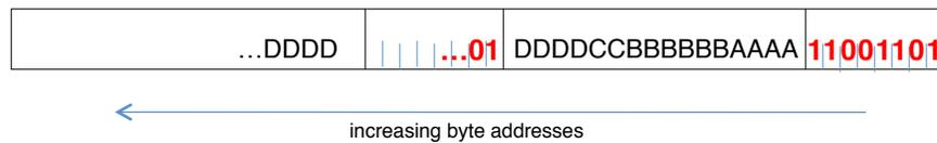
Figure 6: Storing four integers (0xAAAA, 0xBBBBBB, 0xCC and 0xDDDDDDDD) in varint-G8CU format. The last two bytes of the fourth integer carry over to the subsequent data block, and its descriptor bits carry over to the subsequent descriptor byte.
